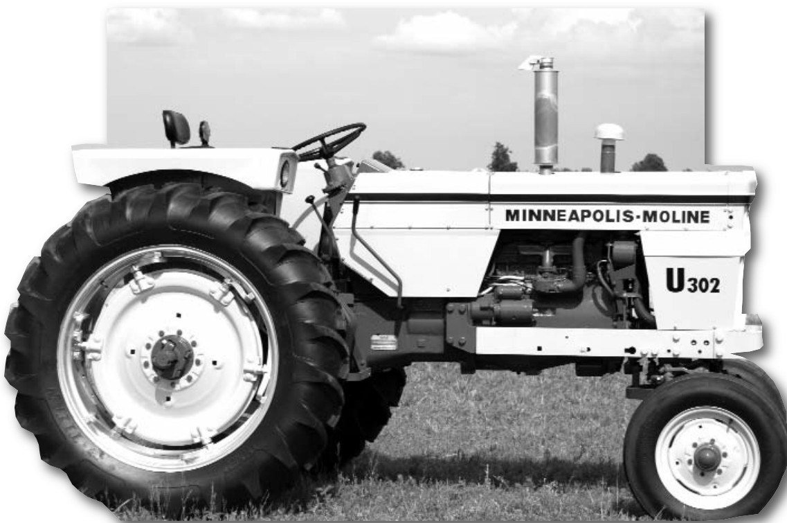
This 1968-69 U302 Minneapolis Moline had an original purchase price of $6,000. It was later purchased at a farm sale in Illinois by Bill Anderson, AKA Cousin Carl, who had it overhauled and totally restored to the original condition by Richard Moldenhauer. Weighing 5,500 pounds, this model was built from 1964 to 1970. It has a 220A-4 engine, 4 Cy. HP drawbar and 56 HP PTO. Cousin Carl will be participating in the Antique Tractor Ride with this tractor.
